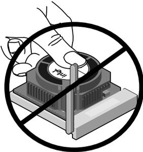
Don't apply pressure to the center of the fan.
