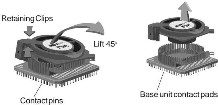
5. Hold the fan at an approximately 45-degree angle, and align the fan assembly over the base unit, starting with the corner opposite the retaining clip. Take special care to align the contact pins on the fan assembly to the three pads on the base unit.
