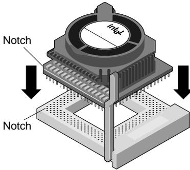
Once the pins and pin holes are properly aligned, gently insert the processor into the socket. Don't use force to insert the processor in the socket.
