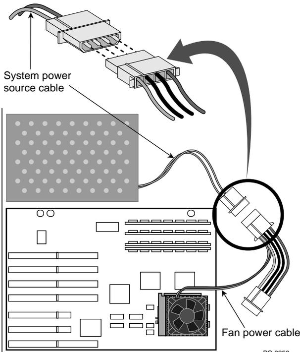
After unplugging the fan power cable from the computer power source, fold the computer power source cable out of the way.
