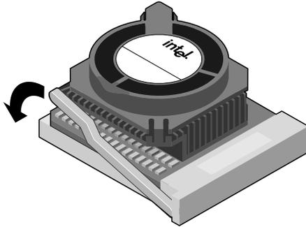
Once it is locked in place, the OverDrive processor with MMX technology should fit snugly in the socket.
